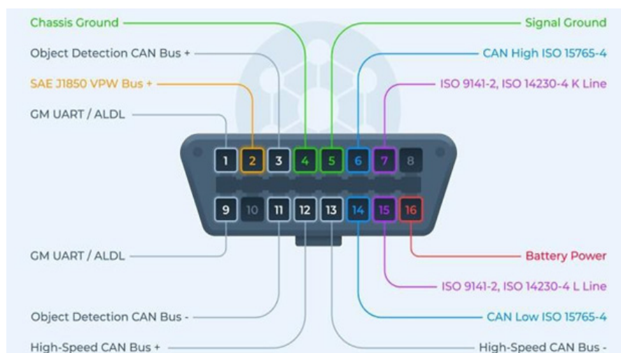
Figure 2. OBDII port pin designation with one or two CAN buses (9)
