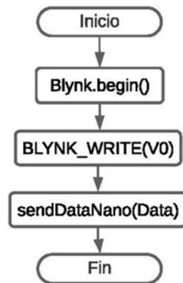
Figure 11. Flowchart for monitoring changes in virtual variables
